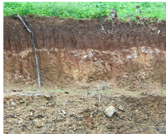
Fig.7. Weathering profile formed over Archean rocks of Dharwar Craton in southern India. The dark brown layer immediately below the vegetation is soil and below it is the saprolite followed by partly weathered bed rocks dark grey in color. The depth of the above profile is about 4 m.
