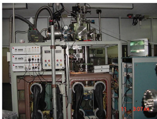
Fig.4. Photograph of Laser-ROTF-MS in vertical configuration [12]
