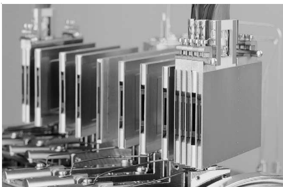
Fig. 3: Multicollector movable faraday cup arrays, and miniaturized ion counters identical in size to Faraday detectors mounted on the high mass side (for U on the left) and low mass side (for Pb extreme right).
